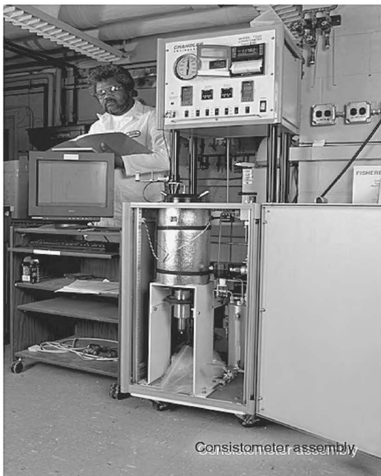
Typical consistometer assembly.
